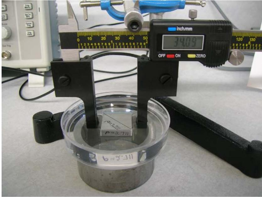
Figure 1-7. Solid sample placed between the transducers.
